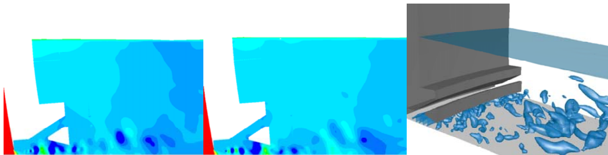
Figure 8 Static pressure at domain's midsection and isosurfaces of pressure for 2m distance to bottom and 1m level difference.
