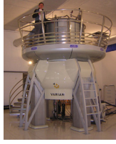
Figure 2: 900MHz, 21.2 T NMR Magnet at HWB-NMR, Birmingham, UK; credit: wikipedia
